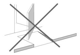
Exposed corners must be rounded or in bevelled angle to avoid becoming hazardous. Platform edges must be clearly highlighted.
